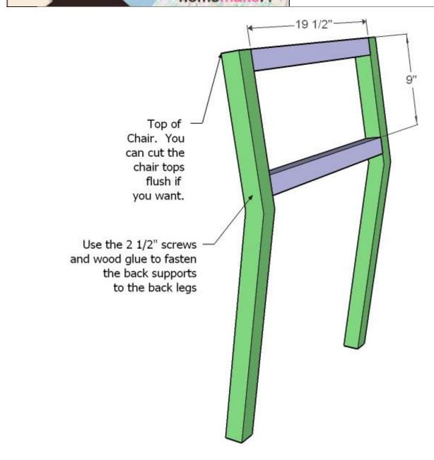
Chair Backs. Build the chair back as shown above. Fasten with  $2^{\prime\prime}$  screws and glue.
