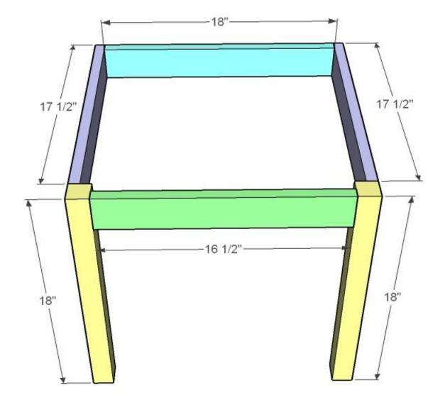
Chair Seat and Front Legs. Build the aprons and front legs as shown above. Start on the back apron and work your way forward. If you have a <u>Kreg Jig</u><sup>m</sup> [3], it would come in super handy here, or else you can just use screws and glue, 2<sup>r</sup> screws.
