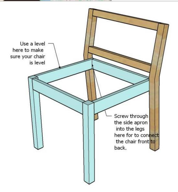
Chair Frame Assembly. Using a level on the side apron, attach the front of the chair to the back, as shown above, using 2<sup>"</sup> screws and glue. You may wish to complete step 5, the seat boards first, but the above diagram illustrates how the chair is assembled.
