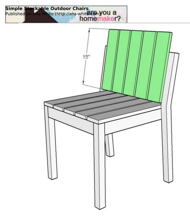
Back Boards. As you did the seat boards, fasten the back boards to the back supports, as shown above.
