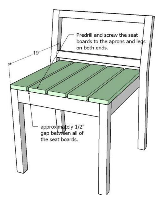
Seat Boards. Predrill and attach the seat boards to the aprons and legs as shown above.
