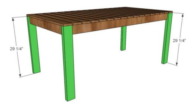
Legs. Screw the legs on with 2 1/2" screws. If you leave the glue off or use bolts, you can make the legs removable.
